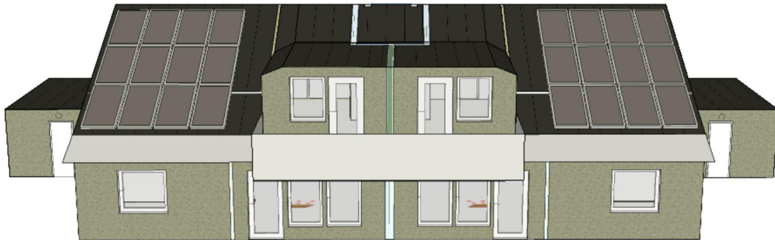
Figure 9. A 3D view of the building modeled in IDA ICE, featuring 7.44 kW p solar PV.
