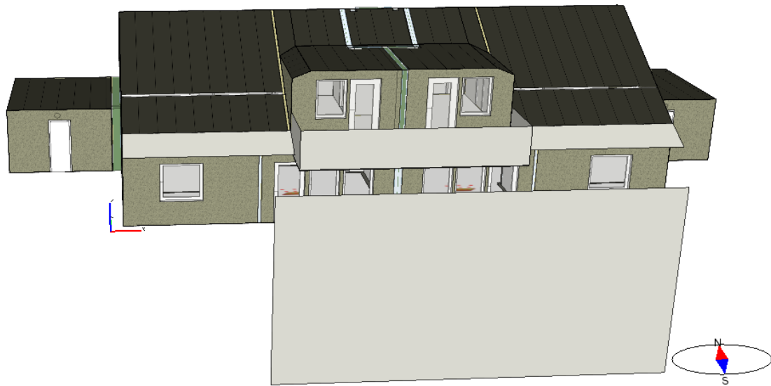
Figure 49. An excessive shading object to assess the effect on building energy demand.
