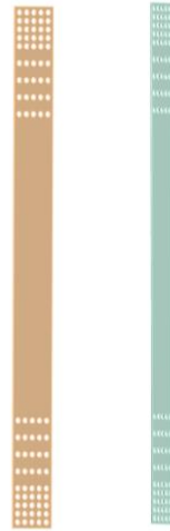
Figure 5.10. Geometry of holed stiffeners with varying stiffness.
